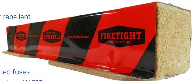
These panels are held together by special pre-tensioned fuses. In the event of a fire and the trigger temperature in the fuse (140°C) is exceeded, these fuses melt, causing the compressed stone wool to expand and completely seal the opening against fire and hot smoke.
